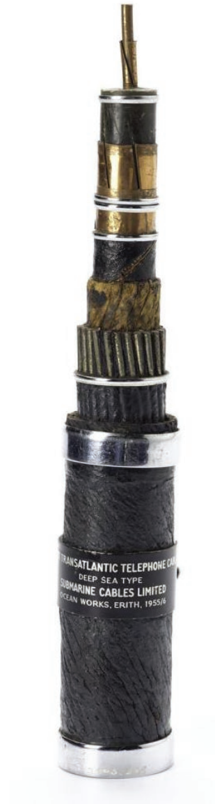
Figure 3.1 Cable sample, TAT-1 deep sea type, 1955. Made by Submarine Cables Ltd (NMS T2003.269), National Museums Scotland
